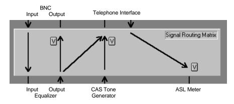
Figure 3: Signal Routing for Test Setup A
