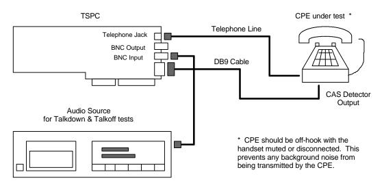
Figure 1: Test setup A
