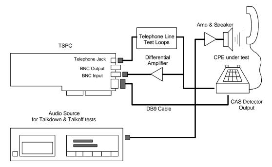
Figure 2: Test setup B
