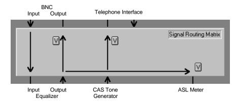
Figure 4: Signal Routing for Test Setup B
